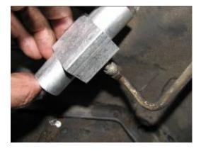
Remove all three caps from the orifice valve and install on the oil return fitting as shown, positioning the larger opening to face the evaporator inlet fitting as shown below.
