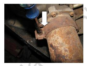
Once the valve is removed, remove the VIR support clamp as shown to the right. This clamp will no longer be used.
