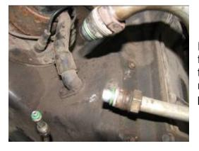
Remove old o-rings from all three evaporator fittings, and make sure all fittings and threads are clean and free of debris. Install new o-rings and lubricate using the oil tube provided.
