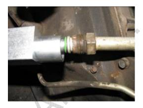
\* SPECIAL NOTE – O-ring hose connections should be tightened to approximately 10-15 pounds of torque. This is generally finger-tight, plus 1/4 turn, but be sure to do a thorough leak test when completed to insure the system is leak free and tighten as needed. Over tightening will result in split o-rings that will result in a leaking hose connection.
